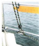
The mainsheet travels from the swivel to a block amidships on the boom slightly behind vertical above the swivel cam cleat. This position allows the mainsheet when running the boom fully out to clear the cabin roof where I have rope clutches and to clear the cabin bulkhead where I coil a halyard and furling line.
