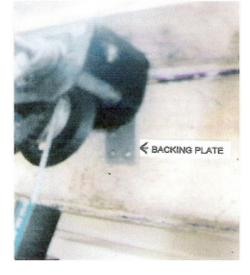
I have my C-22 mainsheet on a Harken swivel cam cleat mounted on the forward cockpit wall.
